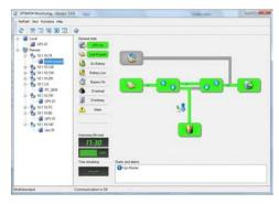
**BLOCK AND FUNCTIONAL DIAGRAMS UPS Monitoring Software** also displays the UPS in block format providing the user with information regarding operating status
