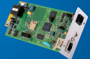
SNMP NetMan 204 card allows management of UPS across LAN using any of the main network communication protocols: TCP/IP; ModBus TCP/IP; ProfiBus DP and BACnet/IP
